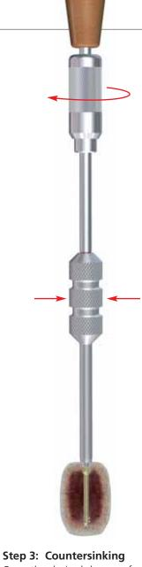
Once the desired degree of compression is reached, the screw is countersunk into the bone with the screwdriver while the compression sleeve is held stationary. During countersinking no additional compression is generated.
