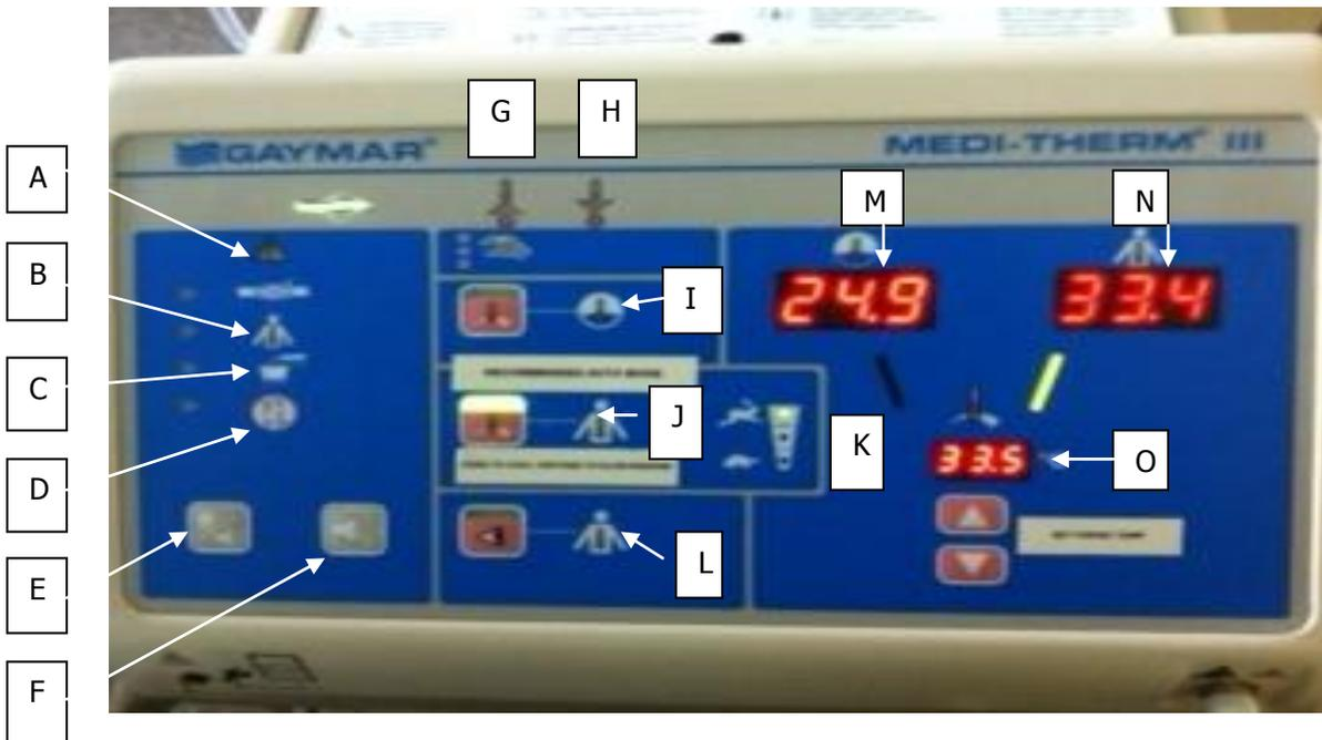
**A. Flow OK-** indicates water is flowing adequately
