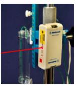
Activate the laser by pressing and releasing red power button (Laser will stay on for 20-30 seconds, then turn off automatically)
