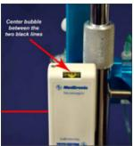
Bubble should rest evenly between the two black lines on the bubble level
