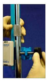
Loosen the black knob on the pole clamp and secure it to the IV Pole
