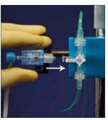
Attach the External Pressure Transducer to the main-system stopcock
