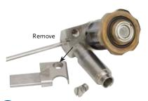
Remove the screw from the Endoscope using a flat head screwdriver.
